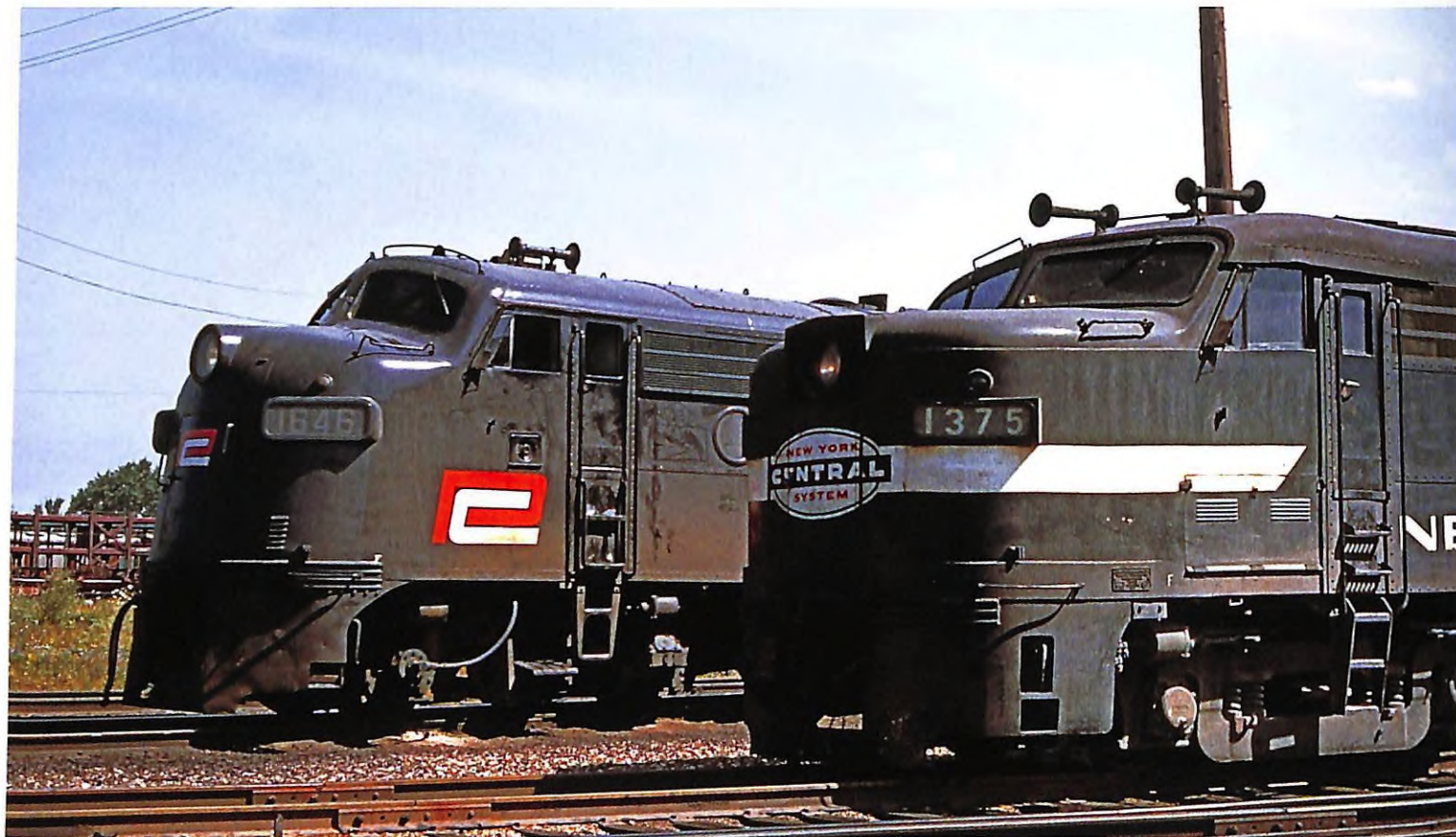
ABOVE: PC F7A 1646 with a red P and ex-NYC FA-2 1375 allow for a comparison of EMD and Alco first-generation cab units in Detroit, Michigan, on July 23, 1968. J.W. Swanberg photo
