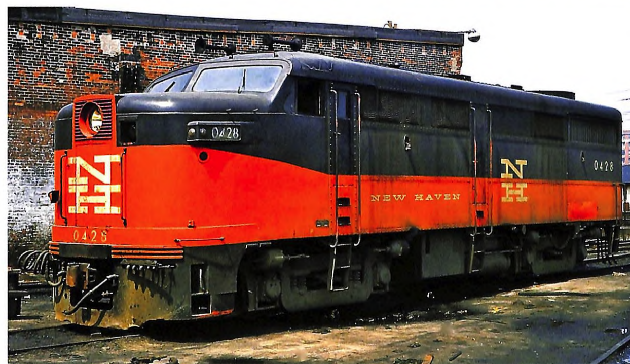
AT LEFT BELOW: Factory rebuilt FA 0428 lays over on a radial track adjacent to the Dover Street roundhouse in South Boston, Massachusetts, sometime in the late 1960s. Spotting features on the ex-New Haven FAs rebuilt by Alco include EMD-style MU hoses on the pilot and the addition of a multiple unit plug to the right of the headlight. Jack Alexander photo, Robert Hughes collection
