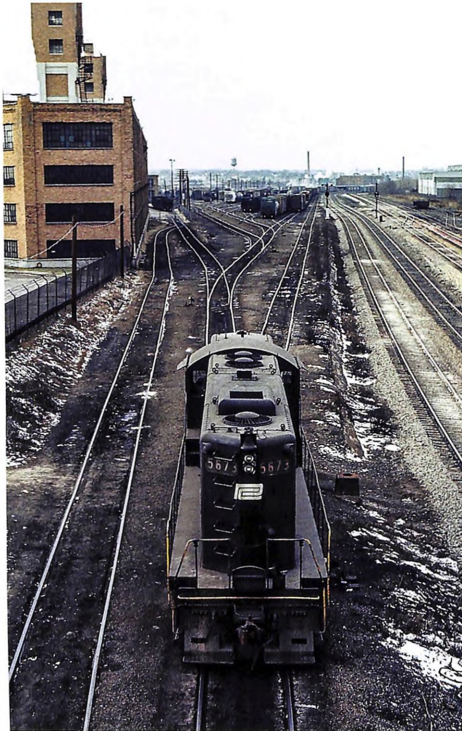
AT LEFT: GP7 5673 pauses on the #103 Secondary Track in this overview of South Akron Yard taken on January 14, 1973. The joint Akron Branch/B&O main tracks are to the left (between the B&O color position-light signals) and the Erie Lackawanna mains are to the far right. Barely visible between the signals is the EL transfer track, where the Ford auto parts cars were spotted for pickup by the EL. Robert Farkas photo
