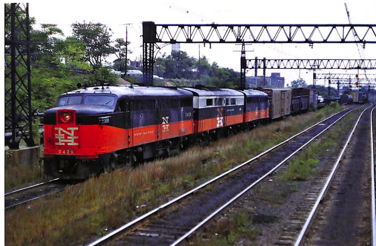
AT LEFT ABOVE: New Haven FA-1 0428, FB-2 465 (in McGinnis colors) and FA-1 0418 are eastbound at New Haven, Connecticut, about to enter the "subway" to Cedar Hill Yard on September 18, 1966. New Haven modified the multiple unit equipment on 465 to permit operation with New Haven's 1956-era road switchers and rebuilt FAs and FBs. J.W. Swanberg photo
