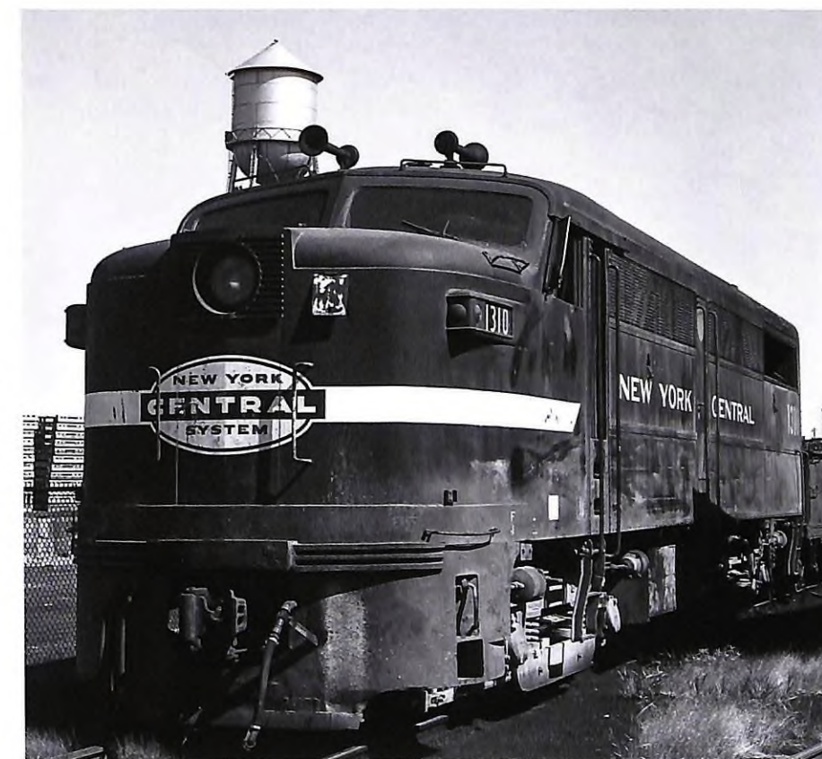
ABOVE: Although wearing New York Central paint and numbered in the FA-2 series, the 1310 at Cleveland, Ohio, (Collinwood) on September 9, 1969, is an FA-1 (former NYC 1033:1) owned by Penn Central. Robert Farkas photo
