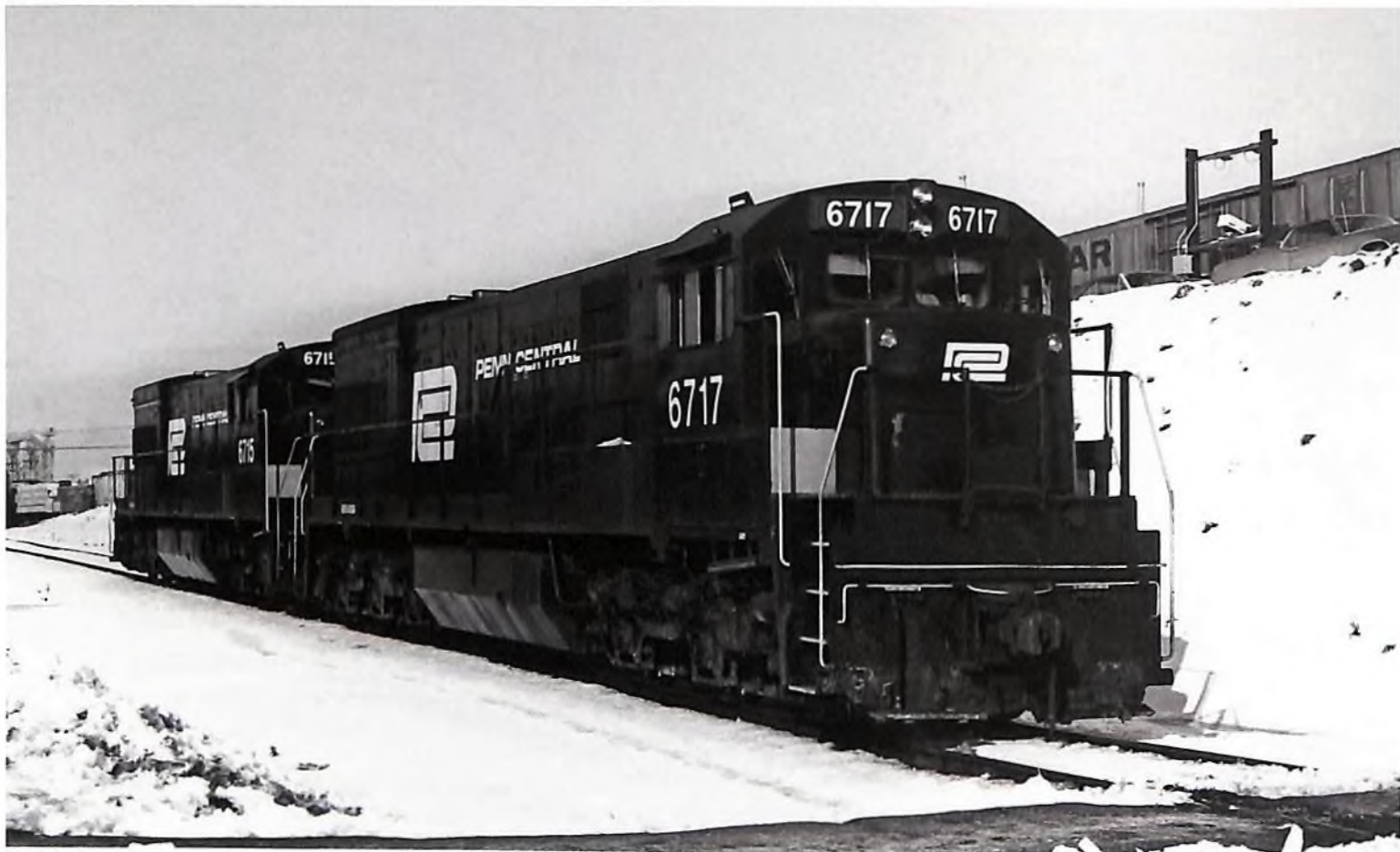
ABOVE: Penn Central took delivery of 19 U23Cs in 1970. Half of them went to Selkirk, displacing the RSD-12s on the hump and in yard puller service. On November 18, 1972, 6715 and 6717 are parked on the Back Track, awaiting their next assignment at the Selkirk hump. James Jensen photo, Kevin EuDaly collection
