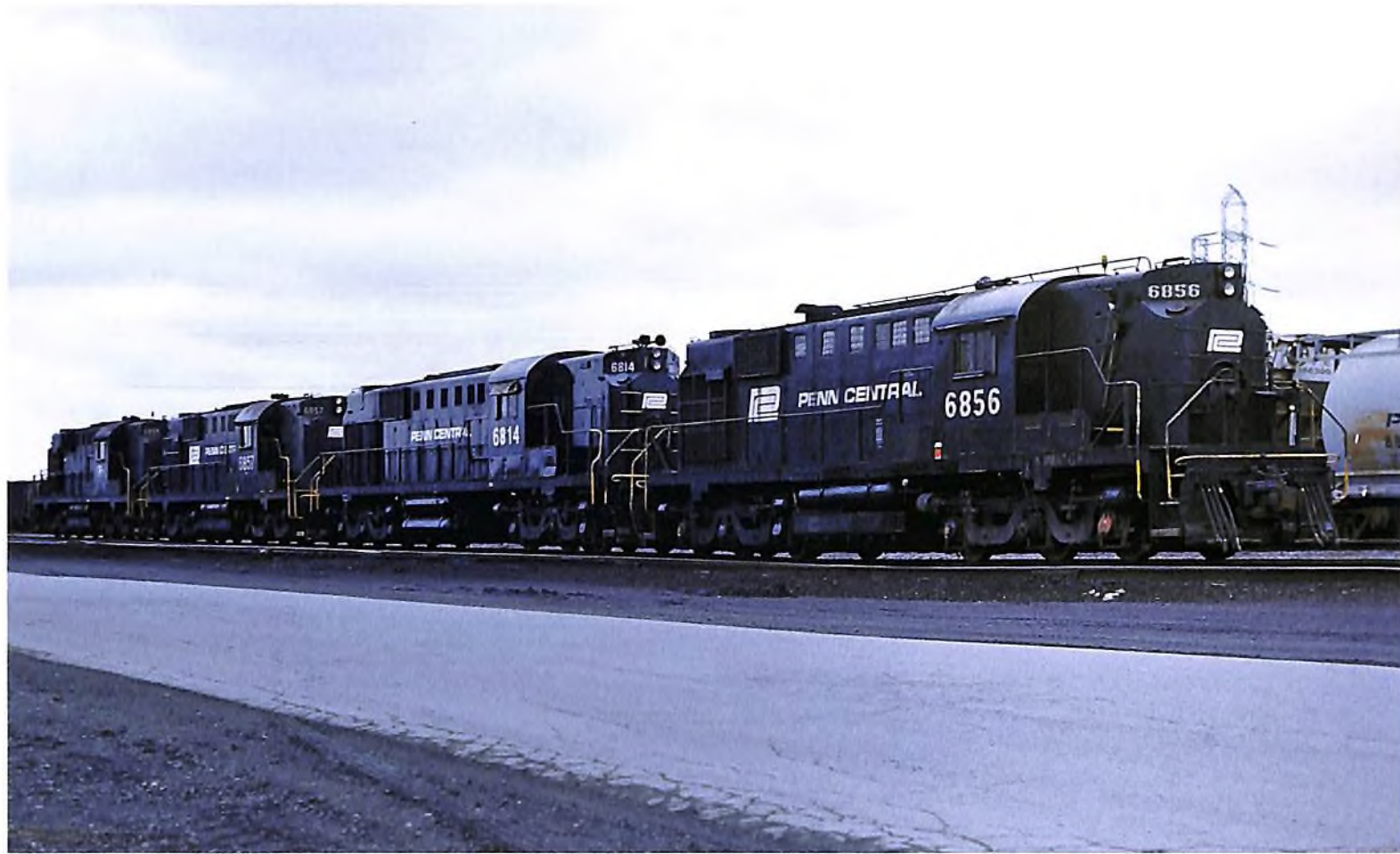
ABOVE: Penn Central concentrated their small fleet of RSD-12s and RSD-15s in upstate New York. The wizards working at the DeWitt diesel shop employed all sorts of tricks to keep these veterans running. Victor Procopio photo, David P. Oroszi collection
