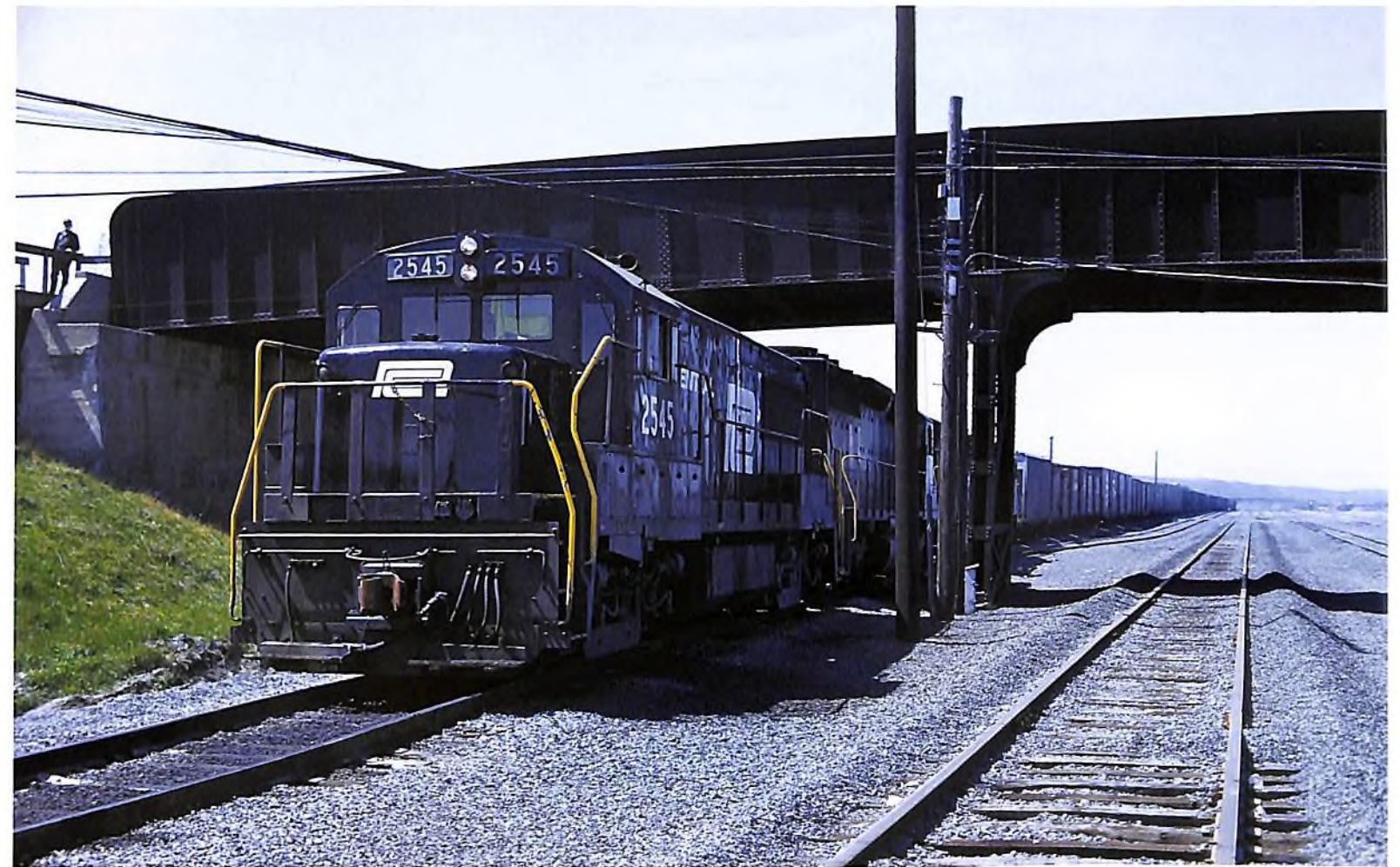
ABOVE: U25B 2545 waits for clearance on Track 11 to depart the Selkirk Yard receiving yard in May 1968. The rebuild of Selkirk Yard, a key pre-Penn Central project, is almost complete — note the piles of fresh ballast. J.W. Swanberg collection
